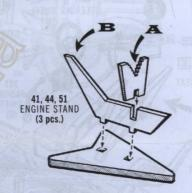
Cement engine stand together as shown above. Display your "extra" engine by cementing its oil pan to point A and transmission to point B.
