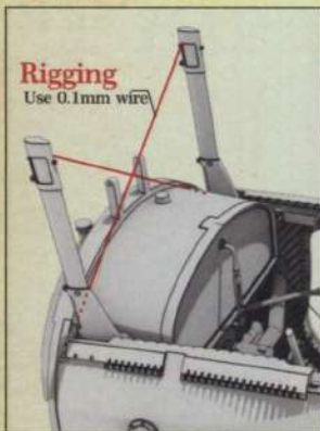
Step 46. Rigging the cabane struts
