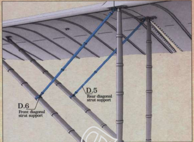
Step 45. Installing the starboard turn struts
