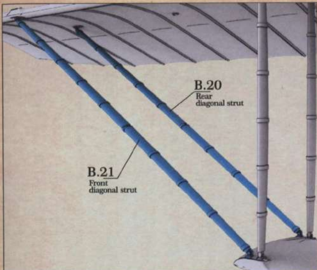
Step 44. Installing the starboard lift struts
