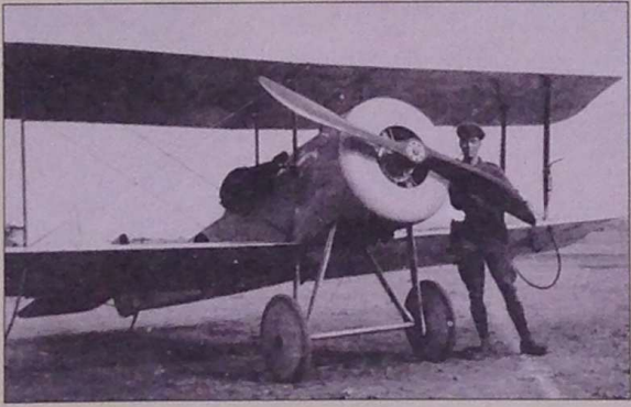
Illustration 1. Scout C 1264, RNAS Francis Donald Holden Bremner served in the Eastern Mediterranean with No. 2 Wing RNAS at Imbros and Thassos. Later on, Sub.Lt. Bremner replaced the Gnome engine with an 80 hp. Le Rhone.
