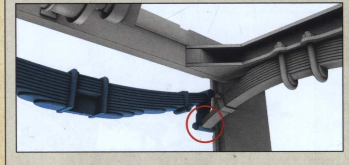
Step 4. Installation of the rear cantilever springs
