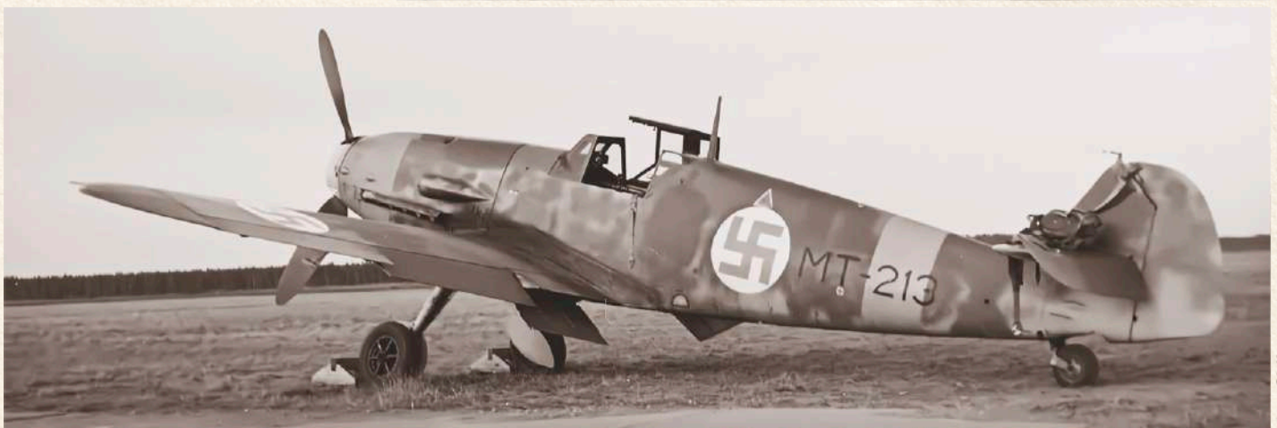
Bf 109 G-4 MT 213 still has the original smaller main landing gear wheels but already sports a larger fixed tail wheel (350x135 mm). This aircraft is part of the marking options included in this kit, but sporting a new camouflage applied after the overhaul.
