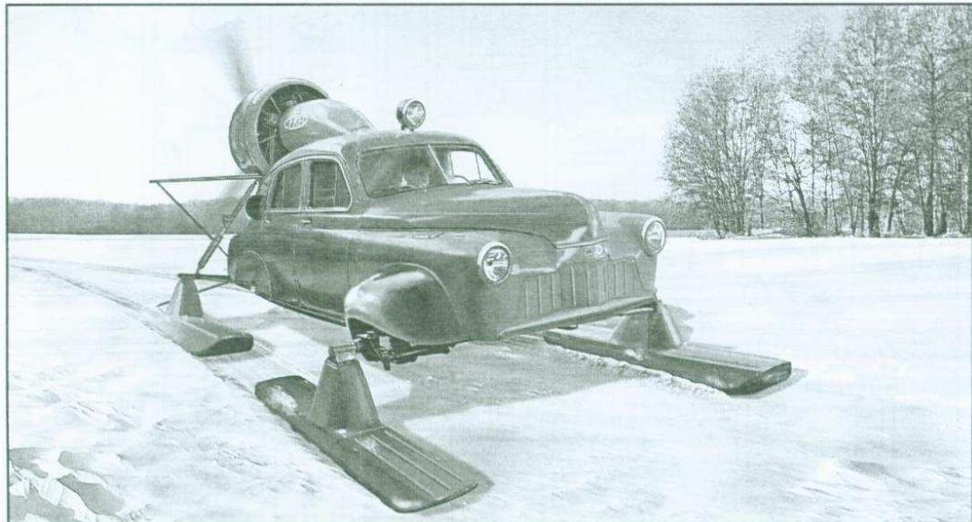
The Sever-2 Soviet snowmobile was built in 1959 at Kamov Design Bureau. It was manufactured at the "Progress" aviation plant. The body of the "GAZ-M-20 Pobeda" with 260-hp AI-14 aircraft engine was mounted on skis. It was turned into fast traffic for the northern areas of the country. The Sever-2 snowmobile was used for such regular services as delivering mail and passenger transportation in Siberia, Russian Far East areas and Kazakhstan.
