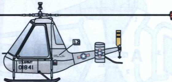
The American Helicopter XH-26 Jet Jeep (known as the XA-8 by its manufacturer) was an experimental tip jet helicopter developed in 1951 by the American Helicopter Company to meet a United States Army and Air Force (USAFA) request for a collapsible and air-droppable observation helicopter.
