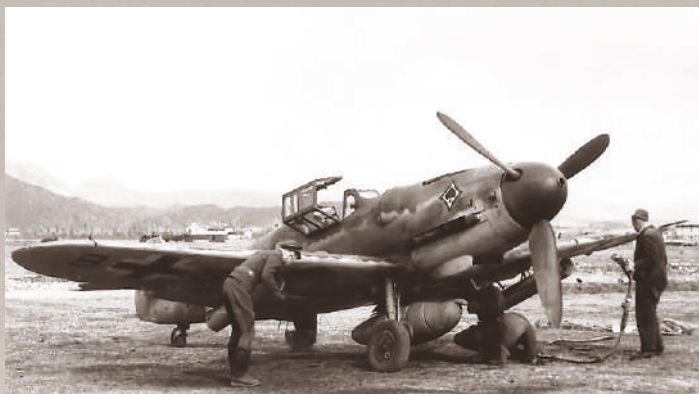
Bf 109 G-6/W of 2./JG 53 "Pik As" with Bordrakete BR 21 cm rockets at the Italian base Maniago in early 1944.
